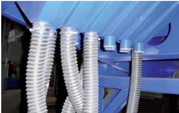
Particle discharge of the screened products is effected via polyurethane hoses. The openings that are closed by rubber caps will be employed if screen decks are upgraded.
