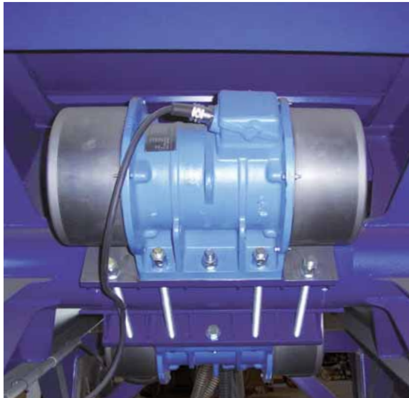
Unbalanced motors generate the linear motion of the multiple-deck screening machine. The motors are clamped onto the drive pipe.
