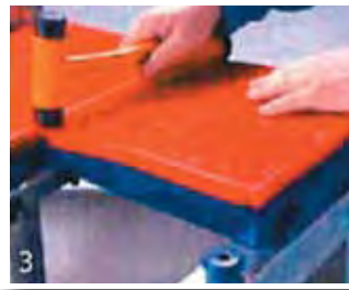
Simple "knock-on" assembly of the screen surface
