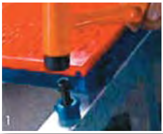
Secure Pin into screen deck
